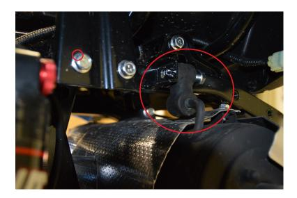
Stage 4 - Loosen the bolt and nut holding the main muffler
