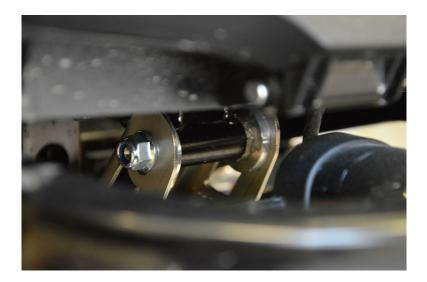
**Stage 8 -** Install the bolts and springs that holds the flange towards the header and tighten them until the bolts bottoms out. Do NOT overtighten these. See picture attached.
